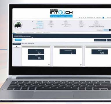
COBO INTOUCH puts in connection COBO devices with a web-server interface. Data are stored in a database and provided to customers via **internet access (by smartphone, tablet and computer)** whenever they need and wherever they are.
